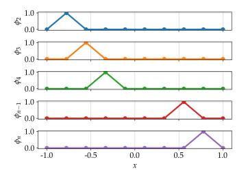
A figure is helpful to illustrate this concept. We will define a set of "hat" basis functions later in this lecture that are depicted in figure **??**. Notice that because they are only nonzero over a small sub-interval of [a, b], many of the inner product terms in *G* would vanish. For example, the only inner products that are nonzero involving  $\phi_2$  are  $(\phi_2, \phi_2)_E$ ,  $(\phi_2, \phi_3)_E$ , and  $(\phi_3, \phi_2)_E$ .
